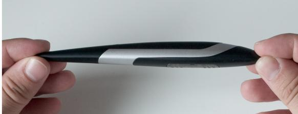
2. Pull firmly the back pen part to separate it from the rest of the pen case
