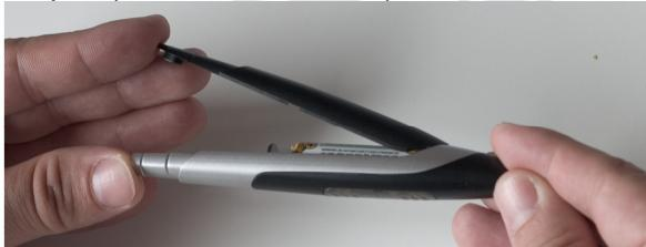
4. Remove the old battery and insert the new one, observing polarity
