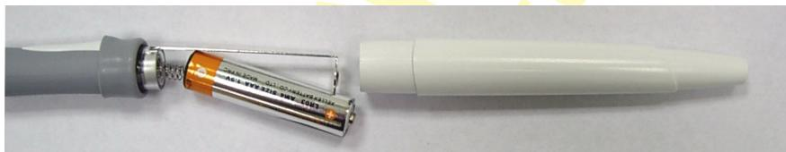
3. Make sure the battery poles are aligned as in the photo below.
